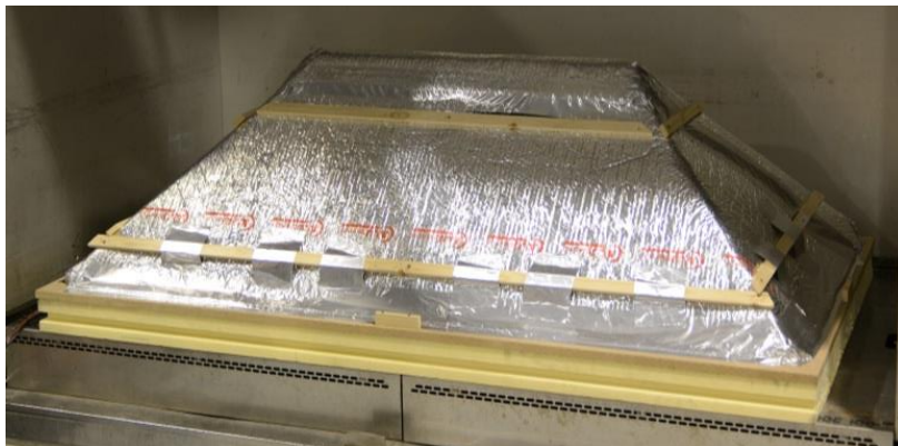
Figure 11 - Structure insulated with 1 layer of Aluthermo Quattro®
