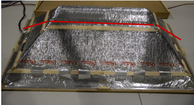
Figure 10 - Insulation with Aluthermo Quattro®
