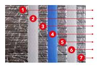
A film of pure aluminium, 30 microns thick, treated against oxidation A layer of bubbles of dry air enclosed in fire-retardant polyethylene A film of pure aluminium treated against oxidation A foam of fire-retarding and waterproofed polyethylene A film of pure aluminium treated against oxidation A layer of bubbles of dry air enclosed in fire-retardant polyethylene A film of pure aluminium, 30 microns thick, treated against oxidation
