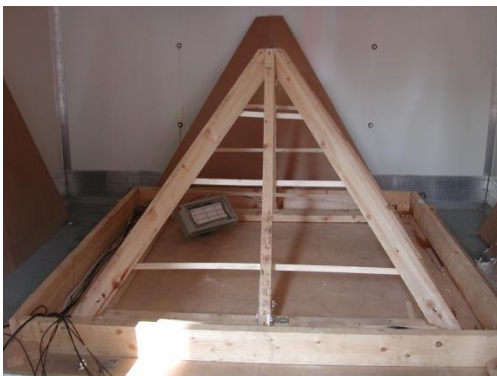
Fig. 1 Roof construction on polystyrene base
